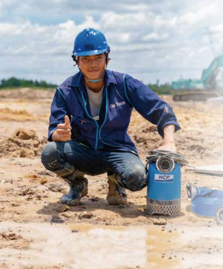
GD-1100 pump can be placed inside the well (diameter 8") for construction dewatering.
